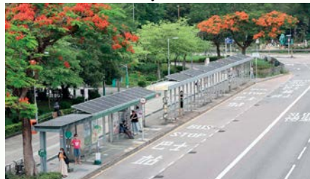
The Kowloon Motor Bus Company (1933) Limited and Long Win Bus Company Limited have installed solar panels on bus shelters to supply electricity for lighting at bus stops
